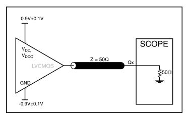
1.8V Core/1.8V LVCMOS Output Load AC Test Circuit
