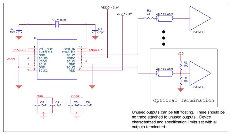
Figure 5. Schmatic of Recommended Layout
