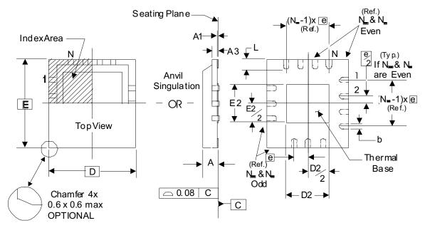
NOTE: The following package mechanical drawing is a generic drawing that applies to any pin count VFQFN package. This drawing is not intended to convey the actual pin count or pin layout of this
