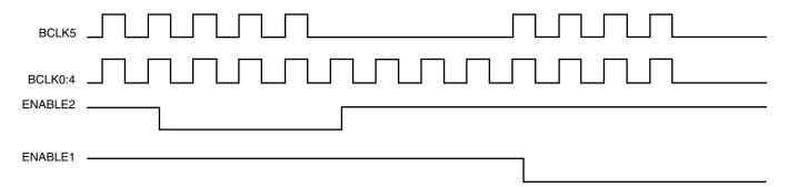
Figure 1. Enable Timing Diagram
