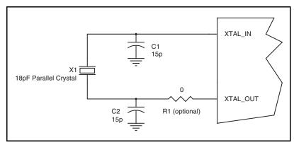
Figure 2. Crystal Input Interface
