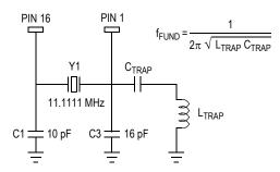
Figure 4. Crystal Oscillator Interface (3rd Overtone)
