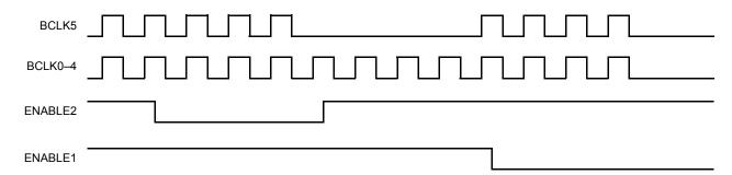
Figure 5. Enable Timing Diagram
