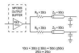
Figure 8. Optimized Dual Line Termination
