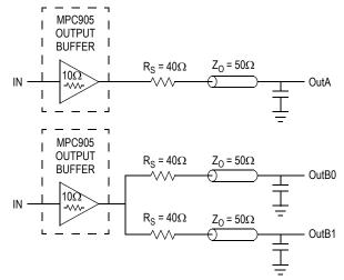
Figure 6. Single versus Dual Transmission Lines
