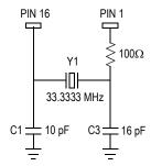
Figure 3. Crystal Oscillator Interface (Fundamental)
