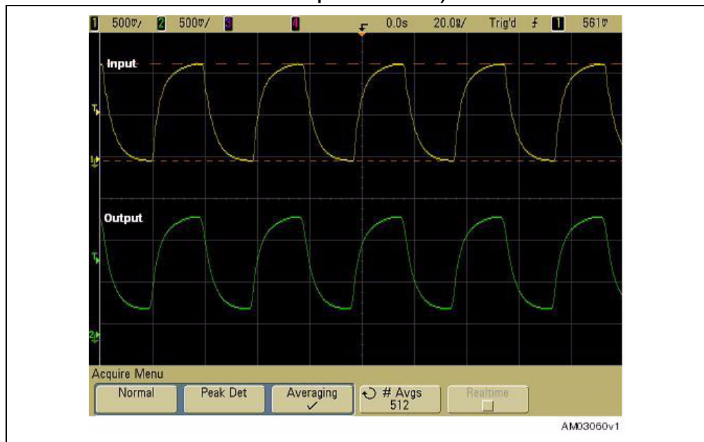
Figure 32. Sine wave input clock vs. output clock (STCD1040, 1.8 V version, 26 MHz sine wave master clock input from TCXO)
