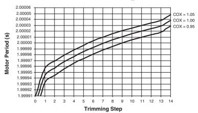
COX means frequency deviation due to production process variations.
