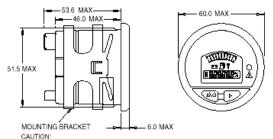
BRACKET IS PLACED OVER GAUGE IN REVERSE FASHION FOR EASE OF SHIPPING BRACKET HAS BEEN DESIGNED TO REMAIN SECURED TO THE GAUGE UPON PROPER INSTALLATION. ONCE INSTALLED CORRECTLY, ATTEMPTS TO REMOVE BRACKET FROM GAUGE MAY RESULT IN DAMAGE TO THE BRACKET.
