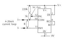
Measuring a 4-20mA loop current.
