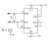
Measuring current. The meter's supply is isolated from the current being measured.
