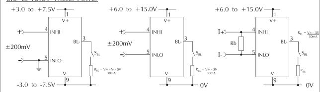
Measuring a single ended input voltage referenced to a split supply, i.e. the input voltage and the meter's power supply share the same OV rail. Ensure solder link LCOM is open.
