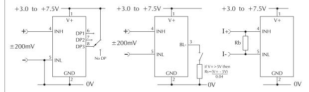
Measuring a single ended input voltage referenced to supply, i.e. the input voltage and the meter's power supply share the same 0V rail.
