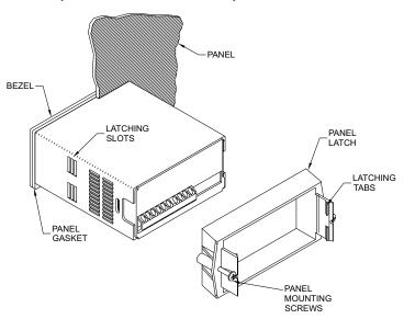
While holding the unit in place, push the panel latch over the rear of the unit so that the tabs of the panel latch engage in the slots on the case. The panel latch should be engaged in the farthest forward slot possible. To achieve a proper seal, tighten the latch screws evenly until the unit is snug in the panel (Torque to approximately 7 in-lbs [79N-cm]). Do not over-tighten the screws.
