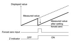
• Press the Up Key while the measurement is being displayed. The displayed value will be shifted to 0 and measurement will be continued.
