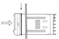
Fit the adaptor into the grooves on the left and right sides of the rear case, then push it until it contacts the panel to secure the K3MA-J.
