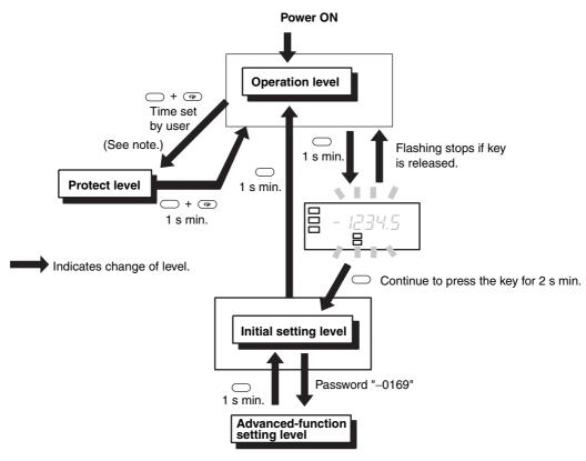
Note: The move-to-protect-level time can be set in the advanced-function setting level.
