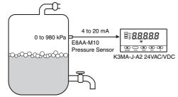
Here, the pressure inside the tank is to be displayed in units of 0.1 kPa.
