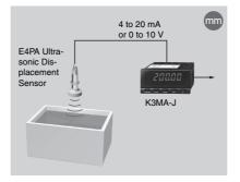
Monitoring liquid level in cleaning tanks
