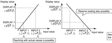
The decimal point can be optionally displayed. When displaying the decimal point, consider the number of digits to follow the decimal point prior to setting the scaling display value.
