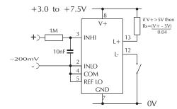
Measuring an input voltage referenced to a floating supply, i.e. the input voltage and the meter's power supply are isolated from each other.
