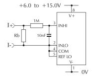
Measuring a current from a circuit which is floating with respect to the DPM's supply, i.e. the current and the meter's power supply are isolated from each other. Ensure solder link LREF is closed.
