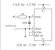
Measuring a single ended input voltage referenced to supply, i.e. the input voltage and the meter's power supply share the same 0V rail. Ensure solder link LREF is closed.
