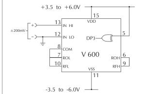
Measuring a single ended input referenced to supply, i.e. the input voltage and the meter's power supply share the same 0V rail.  $\rightarrow$  0V Measuring a current referenced to a floating supply, i.e. the current being measured and the meter's power supply are isolated from each other.
