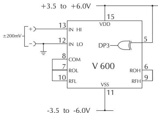
Measuring a single ended input referenced to supply, i.e. the input voltage and the meter's power supply share the same 0V rail.
