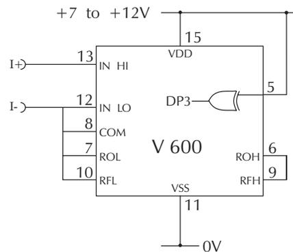
Measuring a current referenced to a floating supply, i.e. the current being measured and the meter's power supply are isolated from each other.
