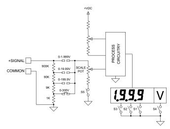
**EXAMPLE**: A relative humidity transducer delivers a 7.0 VDC voltage at a relative humidity of 75%.
