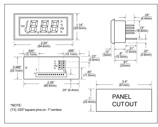
\*Note:Pins 2 & 4 should be tied together for proper operation.
