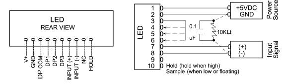
When systems require both power source and signal source to be isolated, please be sure to either directly wire or connect through a  $10K\Omega$  resistor, 0.1uF capacitor, pins two (2) and (8). By doing this errors caused by ground loops will be reduced. The pins that are not being used need to be left open.
