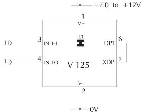
Measuring a current referenced to a floating supply, i.e. the current being measured and the meter's power supply are isolated from each other. Check Link L1 is closed.
