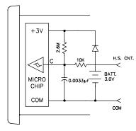
The "H.S. CNT." Input allows the CUB7 to operate at speeds up to 10 KHz when driven by bi-polar outputs or external circuits having an output impedance of 3.3 K $\Omega$  or less. Input drive voltage must be limited to 3 V maximum to avoid damage to the counter. CMOS and TTL Logic outputs can be loaded with a resistor ( $R_L$ ) to limit drive voltage, or a voltage divider can be used as shown for the PNP O.C. Transistor output.
