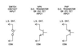
Reed switches, mercury wetted contacts, snap action limit switches, and silver alloy relay contacts with wiping action are usually satisfactory for generating count input signals. Motor starter contacts, tungsten contacts, and brush-type contacts should not be used.
