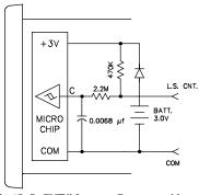
Pulling the "L.S. CNT." Input to Common with a mechanical or solid-state switch increments the counter. The low pass filter (2.2  $M\Omega$  resistor and 0.0068  $\mu f$  capacitor) used with a Schmidt trigger circuit debounces mechanical switch signals. The switch load is 6  $\mu A$  (max. voltage drop 0.5 V) when ON. The OFF-state leakage current must be less than 2  $\mu A$ .
