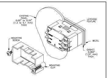
Note: It is necessary to hold the unit in place when sliding mounting clip into position.
