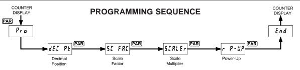
The Totalizer has four programmable parameters which are entered in the sequence shown above, using the front panel push buttons.
