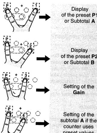
Entry confirmed by pressing the P key briefly or no validation if 15 seconds elapsed with no action
