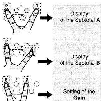
Entry confirmed by pressing the P key briefly or no validation if 15 seconds elapsed with no action
