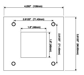
The 1032 panel plate has been designed for use with the M/G/F AXR2, MGF 813 & 11614 Series.
