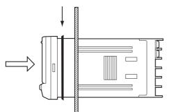
**3.** Fit the adaptor into the grooves on the left and right sides of the rear case, then push it until it contacts the panel to secure the K3MA-F.
