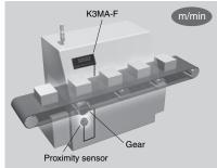
Monitoring line speed for a reflow furnace
