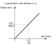
When displaying a flowrate (e.g., in l/min or l/h), make the scaling settings after confirming the I/O characteristics of the flowrate sensor. There are flowrate sensors that output analog signals. If this kind of flowrate sensor is used, consider using the K3MA-J.
