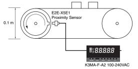
Here, the conveyor belt feed speed is to be displayed in units of 0.1 m/min.
