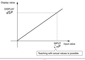
Instead of setting by inputting with the a Up Key and b Shift Key, current values can be input as scaling input values for teaching. This is useful for making settings while checking the operation status of the K3MA-F.
