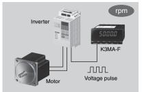
Note: If the monitor output from the inverter is analog, such as 0 to 10 V, use the K3MA-J. Monitoring conveyor speed
