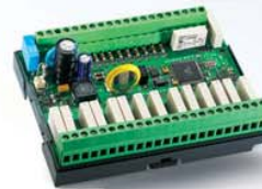
Extended bare board Millenium 3 with 16 relay outputs
