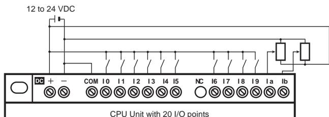
**Note:** When connecting an analog input device, always connect the negative side to the COM terminal.
