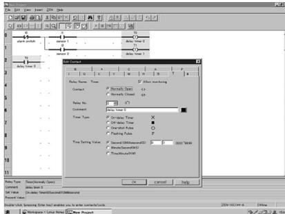
**Note:** The Edit Input Dialog Box is displayed when an input bit is inserted. Timer, counter, and other parameter settings are also set in the Edit Input Dialog Box. They cannot be set in the Edit Output Dialog Box.
