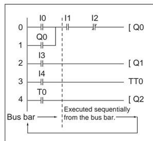
ZEN executes the entire ladder program (up to 96 lines) from the first to last line at one time. Each row is executed in order from left to right starting from the left bus bar.
