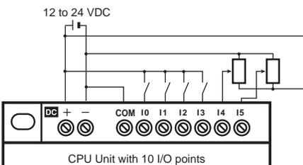
**Note:** When connecting an analog input device, always connect the negative side to the COM terminal.
