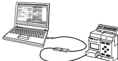
**Note:** For notebook computers that do not have an RS-232C serial port, connect the computer to the ZEN by connecting an OMRON CS1W-CIF31 USB-Serial Conversion Cable to the ZEN-CIF01 Connecting Cable.
