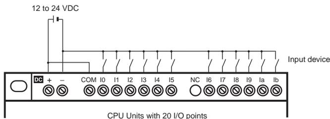
**Note:** When connected to the positive (+) common, 1a and 1b cannot be used as analog inputs.
