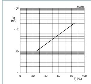
Fig 2. Reverse current as a function of junction temperature; maximum values.
