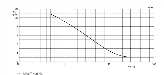
Fig 1. Diode capacitance as a function of reverse voltage; typical values.
