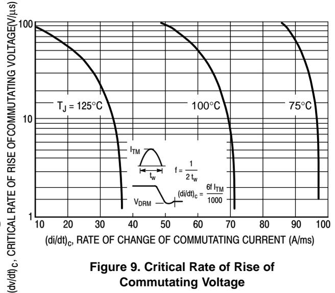
Figure 9. Critical Rate of Rise of Commutating Voltage
