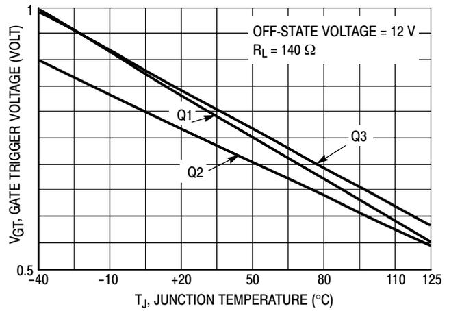
Figure 7. Gate Trigger Voltage versus Junction Temperature
