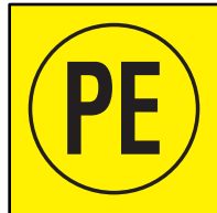
PESC*-PE Protective conductor
