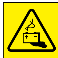
PESC*-BT Warning of battery hazards
