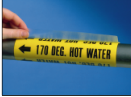
2. Wrap marker around the pipe. The marker will completely encircle the pipe for 360° visibility. Be sure the directional flow arrows are pointed in the proper direction.
