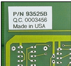
Circuit board labeling
