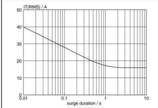
Fig.5. Maximum permissible repetitive rms on-state current  $I_{T(RMS)}$ , versus surge duration, for sinusoidal currents, f = 50 Hz;  $T_{mb} \le 99$ °C.
