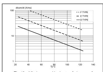
Fig.12. Mimimum, critical rate of change of commutating current  $dI_{com}/dt$  versus junction temperature,  $dV_{com}/dt = 10V/\mu s$ .
