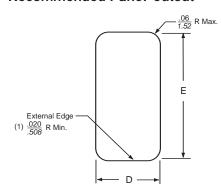
Note: The external edges (installation side) on the "D" sides of the cutout should have a minimum .020" radius. For optional retention against extraction, the corresponding inner edge should be sharp, without paint or coatings. Edge coatings, including anodization are also discouraged for good shield contact.
