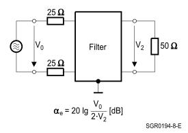
Symmetrical measurement circuit with  $Z_{\text{\tiny L}} = 50~\Omega$
