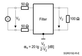
Symmetrical measurement circuit with  $Z_{\text{L}}$  = 100  $\Omega$
