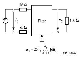
Symmetrical measurement circuit with  $Z_{\!\scriptscriptstyle L} = 150~\Omega$
