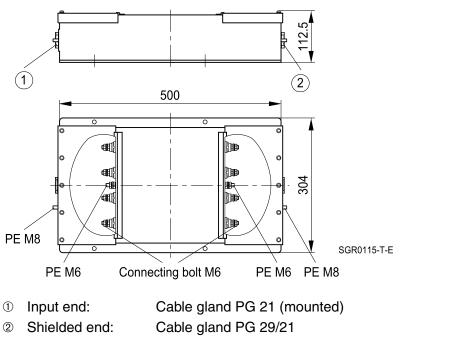
(cable gland PG 29, PG 21 and reducer ring in accessory bag)
