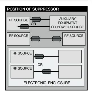
**POSITION OF SUPPRESSOR** The suppressor should normally be located close to the cable termination where it exits the enclosure. Where a cable connects two enclosures containing RF sources, a suppressor on each end may be required. For circuits within an enclosure, a position close to the RF is best. However, other locations along the circuit may work as well.
