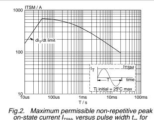
on-state current  $I_{TSM}$ , versus pulse width  $t_p$ , for sinusoidal currents,  $t_p \le 20ms$ .
