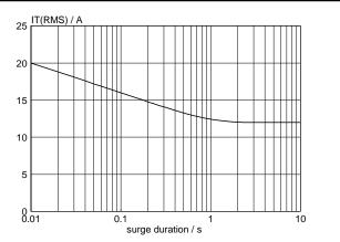
Fig.5. Maximum permissible repetitive rms on-state current  $I_{T(RMS)}$ , versus surge duration, for sinusoidal currents, f = 50 Hz;  $T_{hs} \le 56$  °C.
