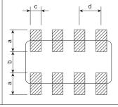
Recommended land dimension for Reflow-soldering (unit: mm)
