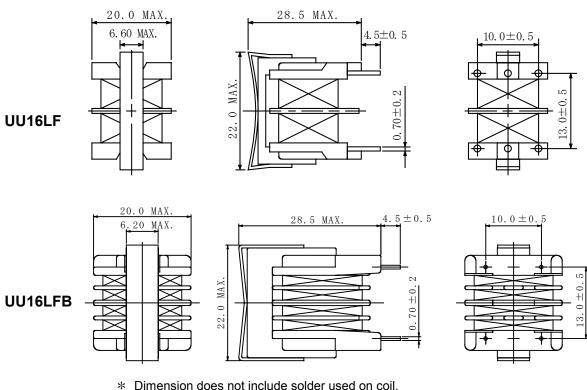
\* Terminal pitch is measured at the base(not from tip of the pin)
