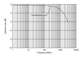
■ Differential Mode Transmission Characteristics (Typ.)
