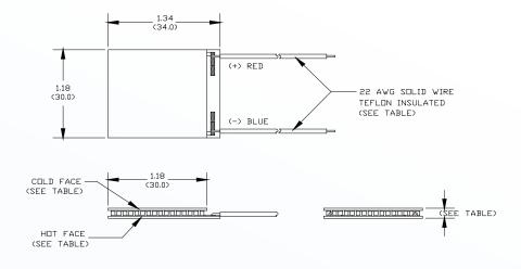
Ceramic Material 96% Alumina Ceramics Solder Construction: 138°C BiSn
