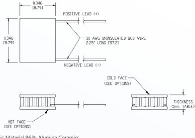
Ceramic Material 96% Alumina Ceramics Solder Construction: 232°C SnSb
