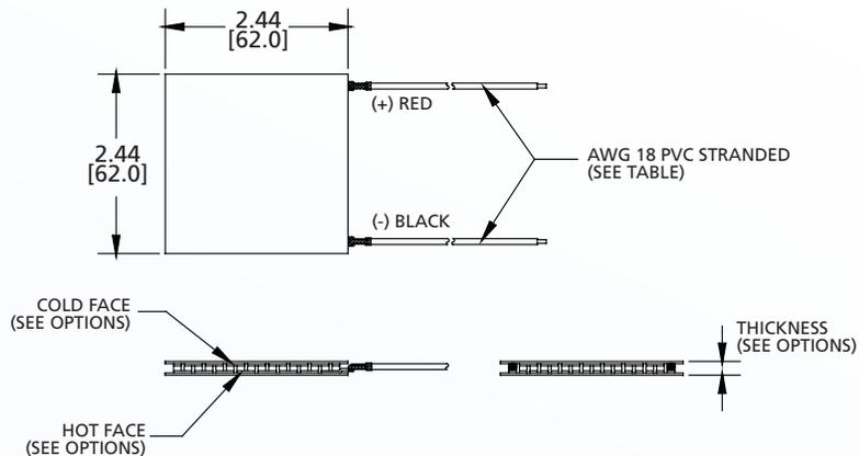
Ceramic Material: Alumina ( $\text{Al}_2\text{O}_3$ )
