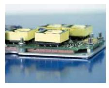
Gap Pad VO Ultra Soft is recommended for applications that require a minimum amount of pressure on components. The viscoelastic nature of the material also gives excellent low-stress vibration dampening and shock absorbing characteristics. Gap Pad VO Ultra Soft is an electrically isolating material, which allows its use in applications requiring isolation between heat sinks and high-voltage, bare-leaded devices.
