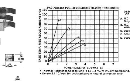
OF CURVES N.C. Horiz. Device Only Freestanding. A. B. N.C. Horiz. & Vert. With Dissipator. C. 200 FPM w/Diss.
