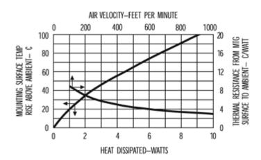
Thermal resistance value is based on a 75°C rise in natural convection
