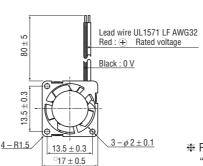
$\divideontimes$  Please reserve  $\phi$  15.9 mm for the vent hole, otherwise "Air Flow" or "Noise" on the specification can't be secured.
