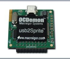
The usb<sup>2</sup>Sprite is a self-powered, cable-less, miniaturized (2.25 in<sup>2</sup>) version of our usb<sup>2</sup>Demon that plugs directly into a board's JTAG/BDM header providing "built-in" debug connectivity. To the user the usb<sup>2</sup>Sprite looks like a USB mini connector sitting on top of the board's JTAG/BDM header. Problems caused by customer installation errors, JTAG cable noise, parallel port incompatibility, and the need for an external power supply are eliminated.
