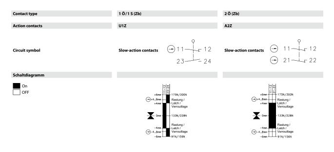
The pulling force data depend on the type of switch used. (SRM...175/SRM...300) Tolerances: Switching point +/- 0.5 mm, actuating force +/- 15 %
