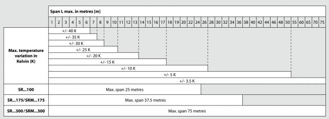
The parameter 100, 175 and 300 in the product designation indicates the force of the springs used in the cable pull switch. It should be noted that a grater actuating force is required for higher spring forces.
