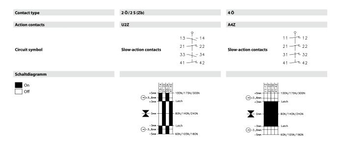
The pulling force data depend on the type of switch used. (SR...100/SR...175/SR...300) Tolerances: Switching point +/- 0.5 mm, actuating force +/- 15 %
