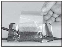
3.11 Starting at top of looped film strip and proceeding downward, seal the loop together until top of mold is closed and the resin fills the mold completely.
