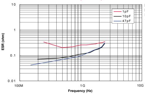
Measurement Equipment Boonton Resonant Coaxial-Line 34A
