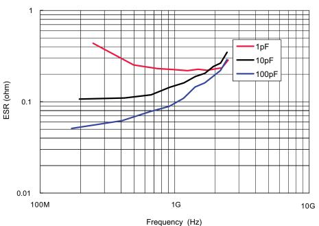
Measurement Equipment Boonton Resonant Coaxial-Line 34A
