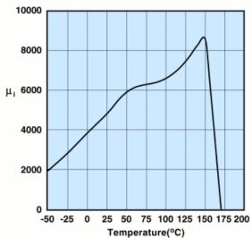
Measured on a 17/10/6mm toroid at 10kHz.
