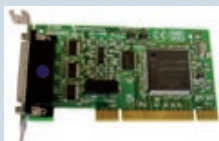
UC-083 uPCI 4xRS232 Opto-Isolated TX RX CTS RTS
