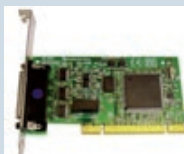
UC-083 uPCI 4xRS232 Opto-Isolated TX RX CTS RTS
