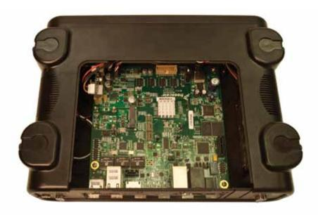
The P1010 RDB platform features 1 GB of DDR3 SDRAM, 32 MB NOR flash and 32 MB NAND flash, and can boot securely from either NOR or NAND flash memory. Other boot options (i.e. SD/MMC, SPI) also supported. It supports three Gigabit-capable ports via an SGMII or RGMII PHYs, as well as a single-port USB and associated PHY.
