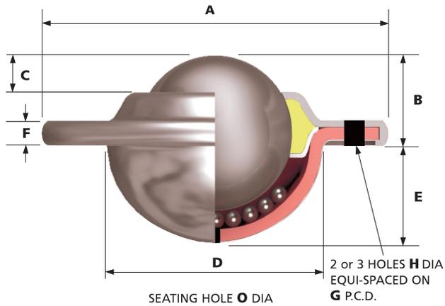
Ball unit Ref. No's 1022 and 1035 with solid steel inner ring (SI) option illustrated with no seal for improved protection from shock loading.
